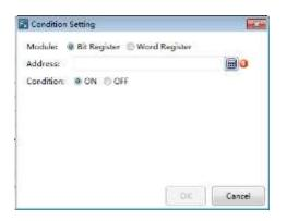
There are two address types: Bit Register and Word Register. The default selection is Bit Register. The logic condition judgment for Bit Register is "ON" or "OFF". The
